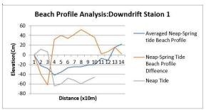
**Figure 8b:** Analysis of effect of Spring Tide on beach sedimentation at downdrift station 1.
