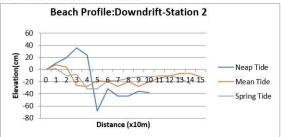
Figure 9a: Beach profiles at down drift station 2 [12].
