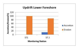
**Figure 7**: Analysis of beach sedimentation and erosion patterns at updrift lower foreshore [12].
