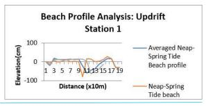
**Figure. 2b**: Analysis of effect of Spring Tide on beach sedimentation at updrift station 1[12].
