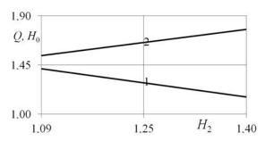
**Figure 4:** Dependence of the cofferdam flow rate Q and the ordinate H0 of the free surface outlet point on the water level in the downstream reservoir H2.
