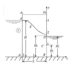
**Figure 1:** shows a rectangular cofferdam with slopes A0A1 and D0B on an impermeable horizontal bed of length L.
